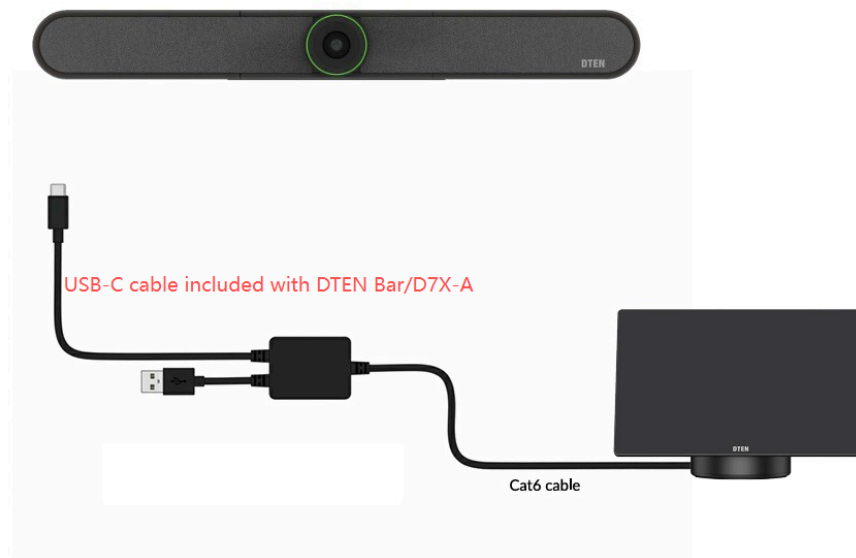
Mate Gen 2 + DTEN Bar connection
